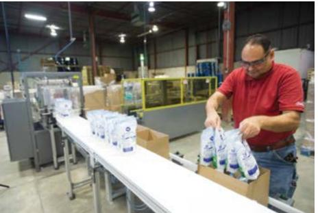
Filled stand-up pouches travel alongside corrugated shipping cases coming out of the Eagle Packaging case-erector to the line operatorm to be inserted inside the boxes.
