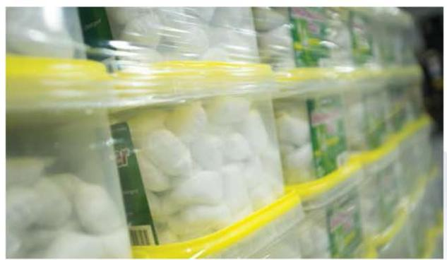
A tight layer of high-strength stretchwrap film helps to keep palleted loads of stacked plastic tubs secure and stable during product transport and delivery to retail customers.
