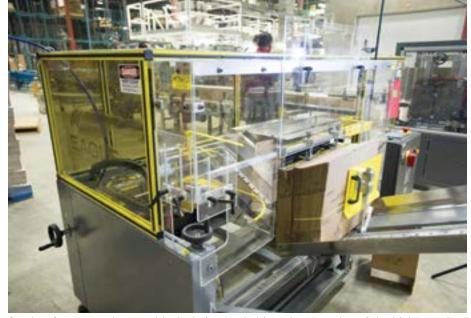
Stacks of corrugated carton blanks being loaded into the magazine of the high-speed, automatic Boxxer T-12 case-erecting machine manufactured by Eagle Packaging.
