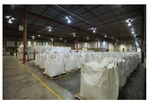
Massive batches of freshly blended and screened dishwasher powder detergent are placed into heavy-duty woven bulk super-sacks in sequential order prior to packaging.
