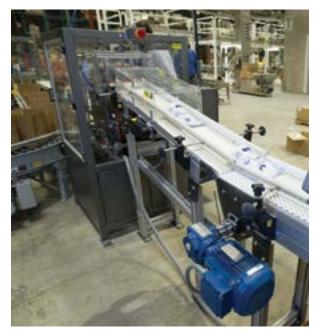
A heavy-duty SEW-Eurodive motor *(foreground)* powers the Speedway conveyors transferring stand-up pouches inside the Eagle Packaging collating machine.
