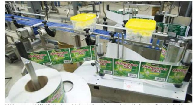
A high-speed model SPM-10 side wipe-on label applicating system manufactured by Speedway Packaging Machinery swiftly applies pressure-sensitive product labels onto the side panels of plastic tubs with exacting placement precision.
