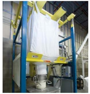
A heavy-duty woven super sack filled with bulk powder detergent blend is prepped up for discharge and processing into monodose, single-use dishwashing detergent tablets.
