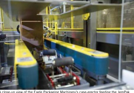
A close-up view of the Eagle Packaging Machinery's case-erector feeding the JemPak packaging lines with corrugated shipping boxes made by Atlantic Packaging Products.
