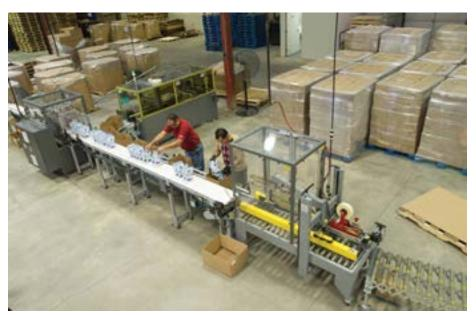
A bird's-eye view of one of the plant's two highly-automated packaging lines utilizing high-speed collating, box-erecting and case-sealing equipment from Eagle Packaging.
